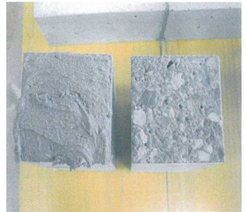
Prism components prior to joining, coated on the left side using BT– Universal Bond
